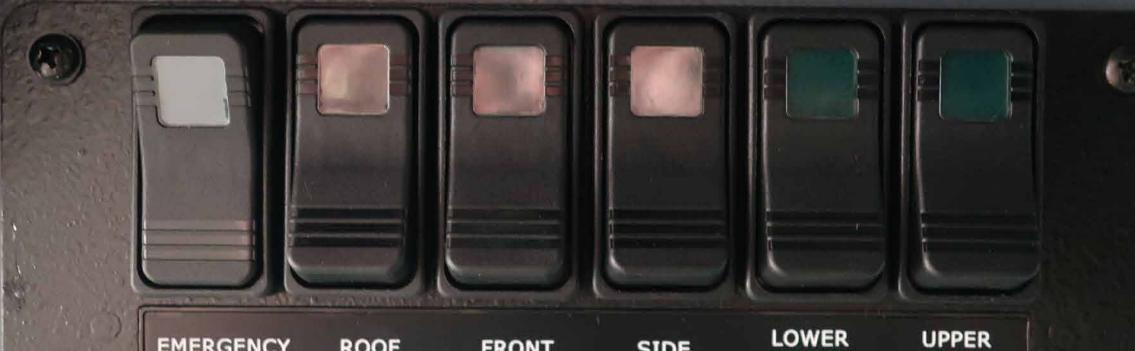
EMERGENCY MASTER ROOF LIGHT FRONT WARNING SIDE WARNING LOWER REAR WARNING UPPER REAR WARNING
