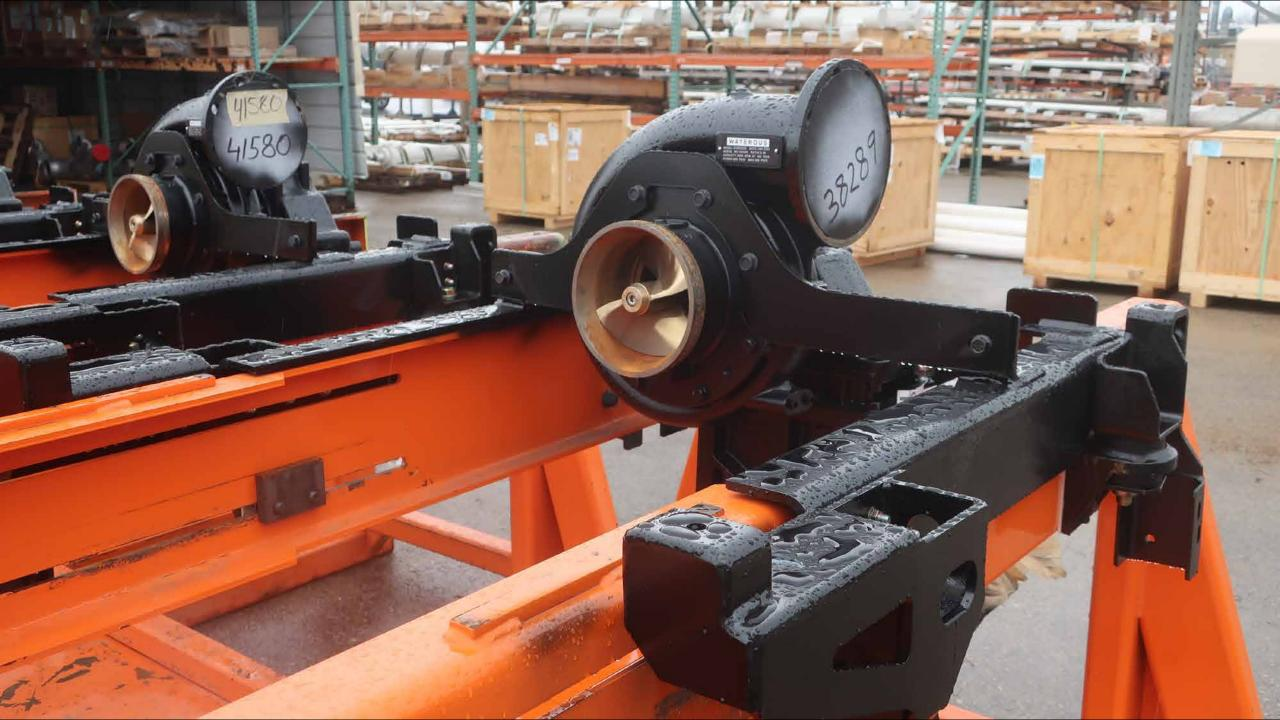
WATEROUS MODEL:S100C22D DATE:JAN-2024 SERIAL NO:181845 RATIO:2.46 CAPACITY:2000 GPM AT 150 PSIG HYDRO:500 PSIG MAX:300 PSIG
